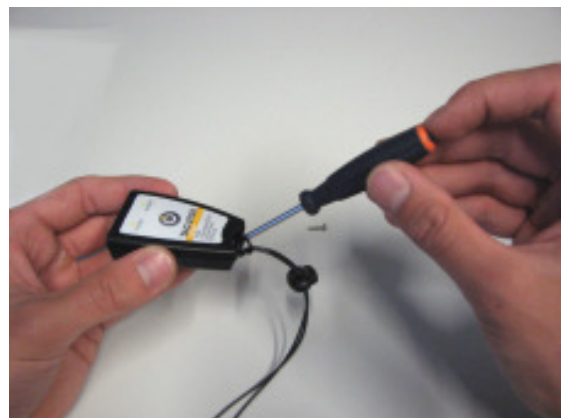
Figure 6. Removal of the covering
