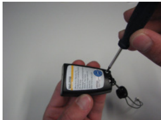
Figure 5: removing the screw on the reverse side of the TAG 2550
