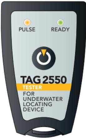
Receives ultrasonic signals between 25 and 50 kHz
