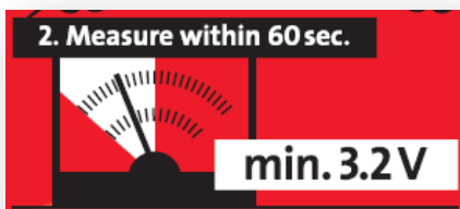
Figure 6: Battery voltage measurement
