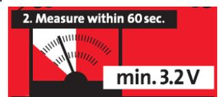
Figure 6: Battery voltage measurement
