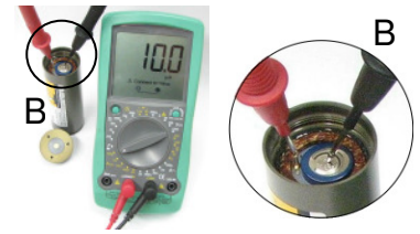
Figure 4: Measurement of electrical consumption
