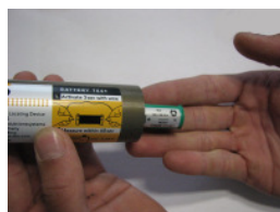
Figure 2: Removal of the battery
