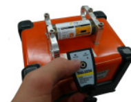
Figure 6: Check the ultrasonic signal with Tester TAG 2550
